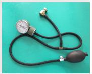
made by DPC. The vent at the back of the housing is unscrewed and the adaptor of the tool is screwed in instead. Pump the balloon gently to a pressure of 40 mmHg. The pressure droop (rate of drop) should not exceed **1mmHg per 10 seconds**. Any droop faster than that will allow water to eventually enter the housing.
