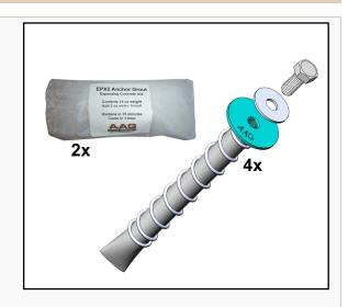
Installation The installation requires drilling a 7/8" hole, 6" deep, into the asphalt and the gravel below it. The grout is supplied as a cement powder. It requires the addition of water to activate it. The hole is filled with the grout and the anchor is dropped in. The anchor is ready for use in 15 minutes .
